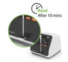
Apply the sample mixture into the sample well of the test device and immediately press the start button.
